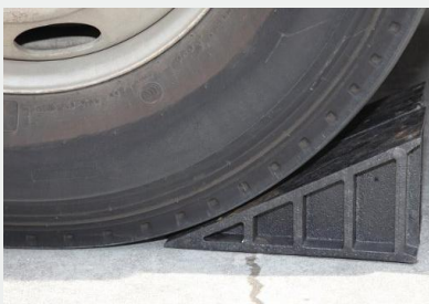
Wheel chocks are in place after parking the vehicle.
